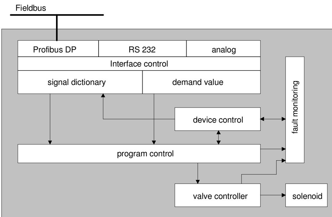
The DP-Slave controller card contains the complete Hardware of the ED1/SD1. This Hardware includes the interface for the Fieldbus and the interface for the parameterisation software PASO. Also included are all digital and analog inputs and outputs as well as 2 solenoid outputs for the cylinder.
