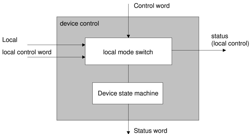
The parameter "Local" indicates the source of the control word acting on the device state machine.
