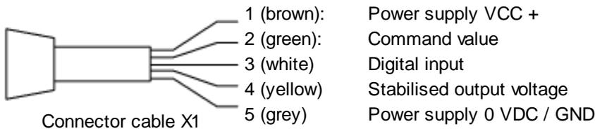
Solenoid connection (only with version with additional solenoid cable):
