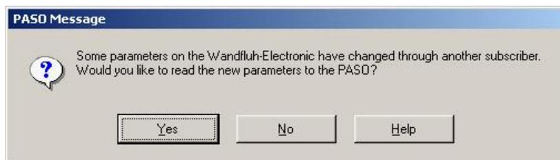
If the answer is "Yes", then the parameters will be read-in from the MD2-Electronics. Possible open parameter windows in the PASO will be closed automatically. If a parameter value will be changed through the fieldbus after the read-in of the new parameters, this message will appear again.
