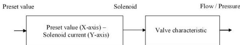
At shipping ex work (default settings) the preset value is transmitted proportionally to the solenoid current (default characteristic). In this case the characteristic "Preset value (X-axis – Solenoid current (Y-axis))" is linear. The same behaviour occurs at any time when the characteristic optimisation is turned off.
