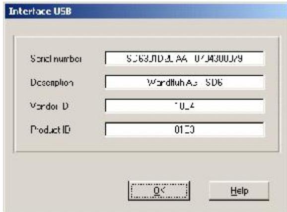
You can see these items also in the OFF-Line mode and without power supply on the SD6 card. If these items are not visible, there is a problem with the USB driver or with the USB connection. To check the USB driver, go through the following steps:
