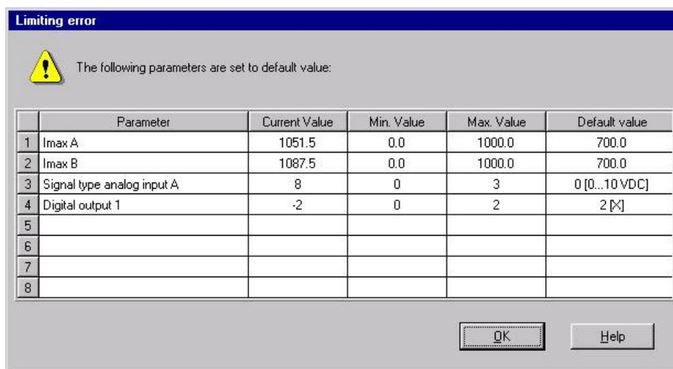
Parameter: Name of the parameter with the limiting value error
