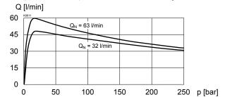
$\Delta p = f(Q)$  Pressure drop volume flow characteristics (I = I<sub>o</sub>)
