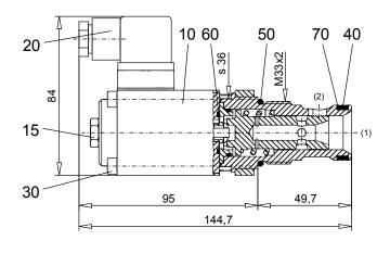
Cavity drawing according to ISO 7789–33–01–0–98
