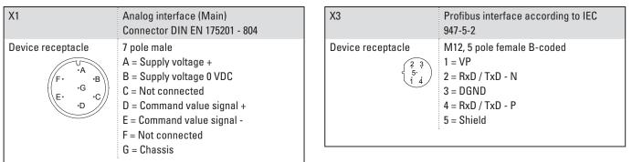
Command value signal: current (D4) or voltage (D2) to specify when placing the order
