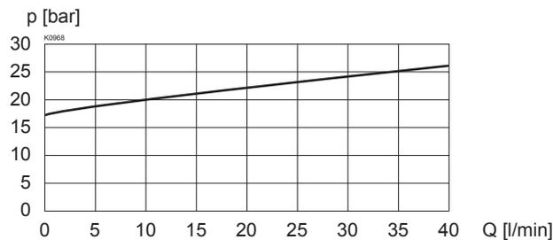
**$\Delta p = f (Q)$**  Pressure drop volume flow characteristics 1 → 3
