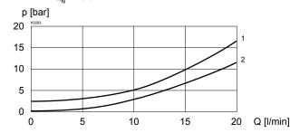
$\Delta p = f(Q)$  Pressure drop characteristic 1 = Flow direction P $\rightarrow$ A 2 = Flow direction A $\rightarrow$ T  $Q_N = 20 \text{ l/min}$
